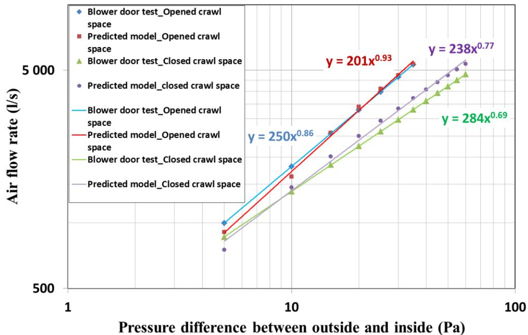
**Figure 2** Blower door results for two cases: the apertures of the crawlspace are opened or closed. Power law relationship between pressure difference (x) and airflow rate (y) are presented for each case.
