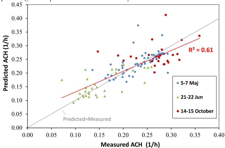
**Figure 3** Predicted (simulated) and measured infiltration rates during 5-7 May, 21-22 June and 14-15 October.
