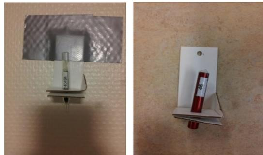
Figure 2: A passive sampler (left) and a tracer source (right)
