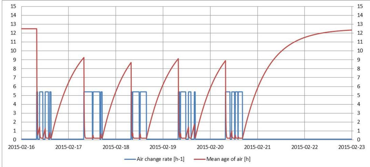
Figure 5: The diagram shows the air change rate (blue, left axis [ $\text{h}^{-1}$ ]) based on the damper positions from Fig. 3 and using the average air leakage ( $0.08 \text{ h}^{-1}$ ) at low operation and  $5.4 \text{ h}^{-1}$  (see text) at high operation. The simulated mean age of the air (red, right axis [h]) using Eq. 6 is shown for the same room and period.
