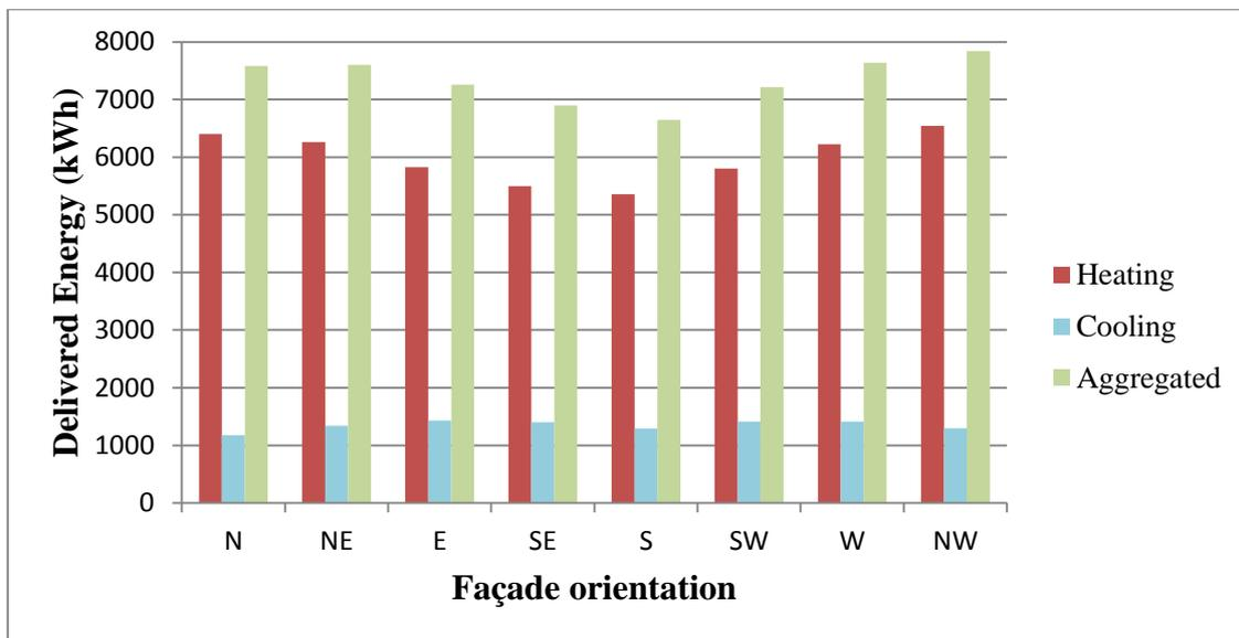
**Figure 4-2.** Energy delivered for heating, cooling and the combination of both for each orientation in Scenario 1.
