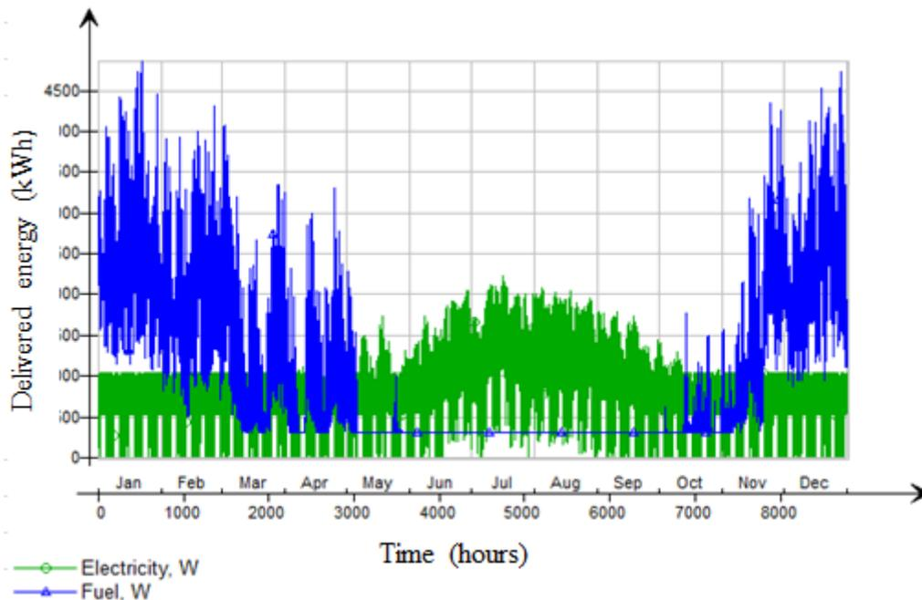
**Figure 3-1.** Electricity and fuel use during the simulation year.
