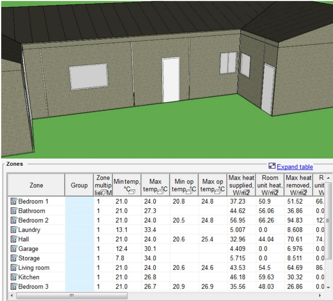
**Figure 2-2.** Screenshots of IDA ICE interface, showing the 3D model of the dwelling (up) and an extract of the simulation results (down).
