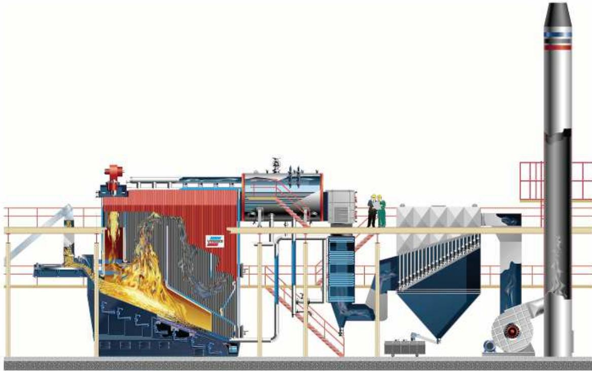
Figure 9: Typical layout of complete boiler
