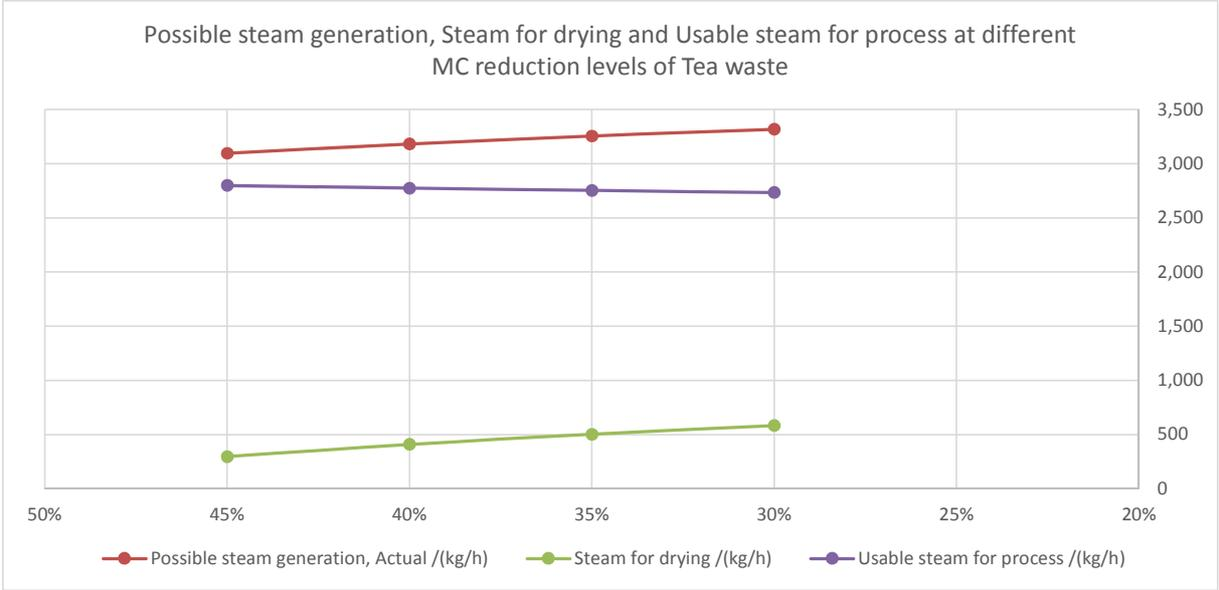
Figure 2: Possible steam generation, steam for drying in rotary dryer and usable steam for process at different moisture reduction levels from 55% MC on wet basis of tea waste
