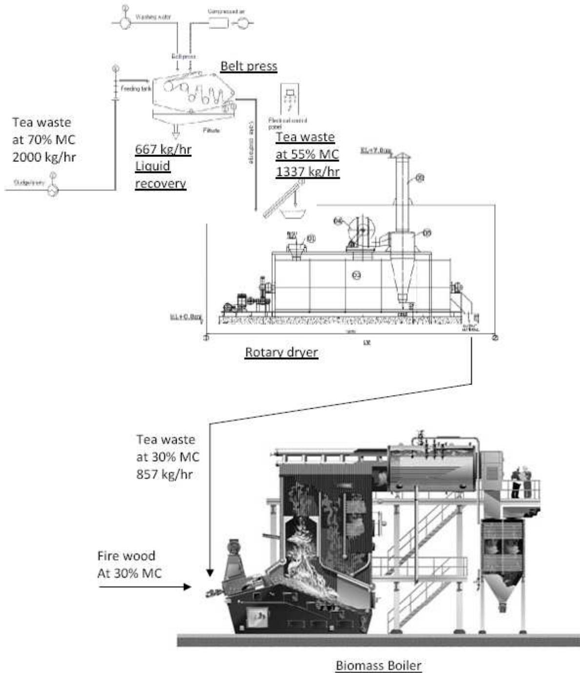
Figure 3: Proposed configuration of plant
