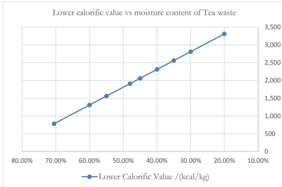
Figure 1: Lower calorific value of tea waste at different moisture content on wet basis
