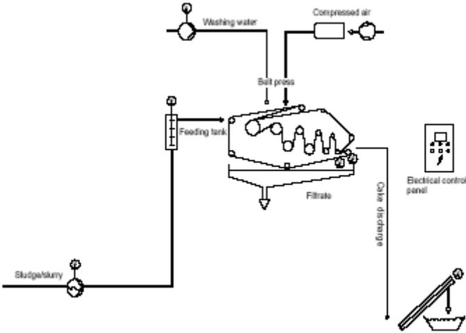
Figure 4: Belt press configuration
