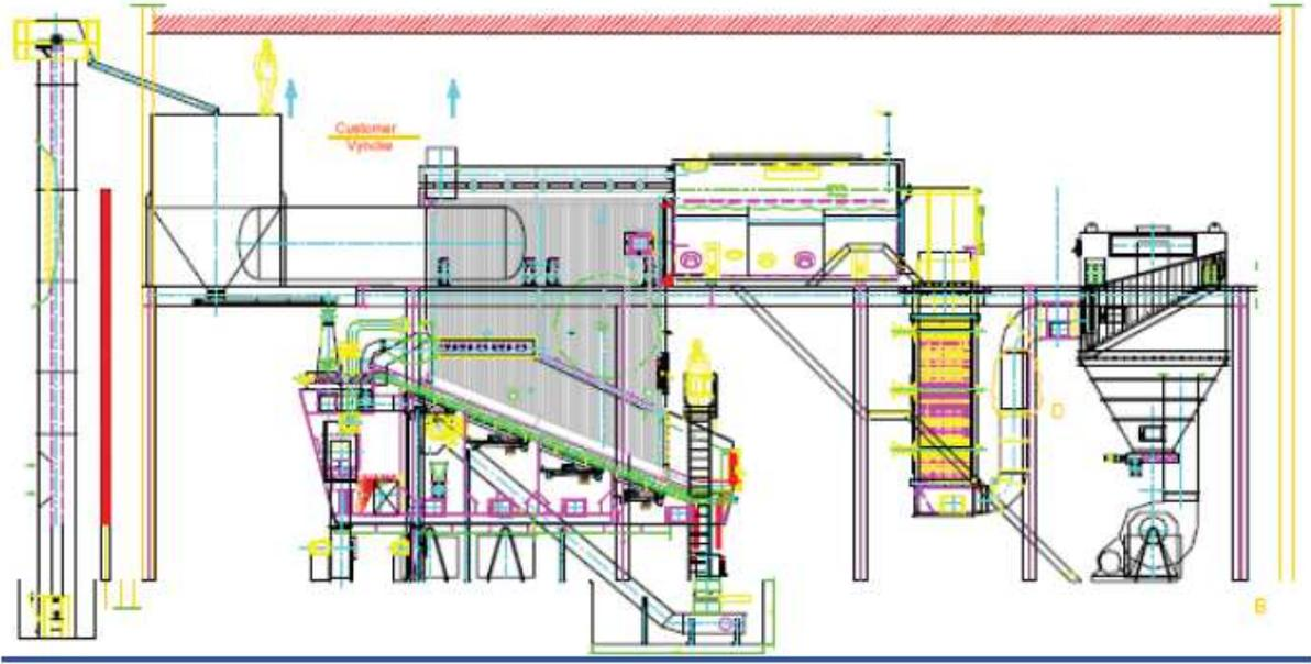
Figure 7: Principal layout of boiler plant (Dynamically air cooled steam grate boiler)
