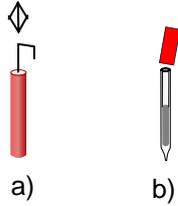
**Figur 2.** a) Adjustable passive tracer gas source b) charcoal adsorption tube used for pumped sampling of PFTs.
