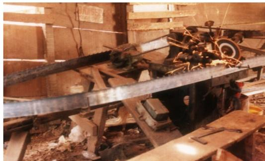
Figure 9, blades sharpening machine, image by author
