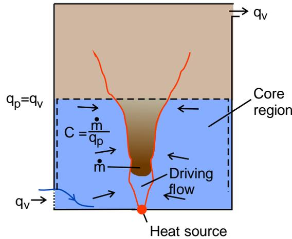
Figure 5. Due to entrainment of ambient ventilation air the dilution capacity is equal to the flow rate  $q_p$  in the plume
