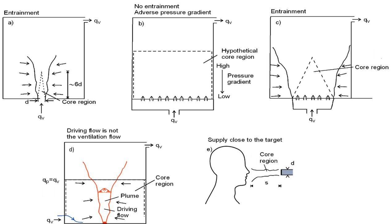
Figure 4. Direct supply of clean air. a-d) expanding the core region, e) Supply close to target
