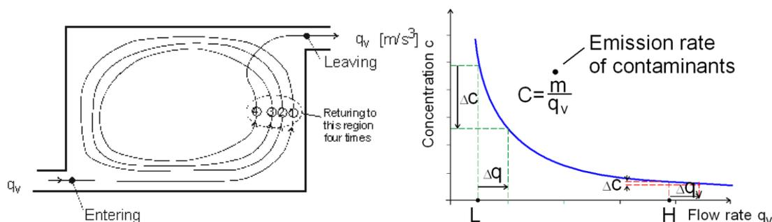
Figure 3. Left: Archetype of a mixing system; Right: Dilution curve (L: Low flowrate H: High flowrate)
