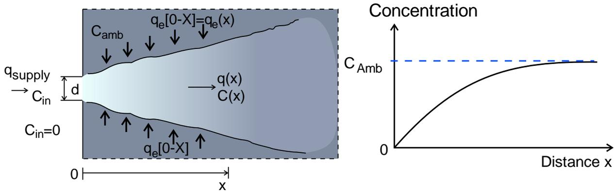
Figure 6. Supply of clean air,  $C_{in} = 0$ , into a room filled with a pollutant of uniform concentration
