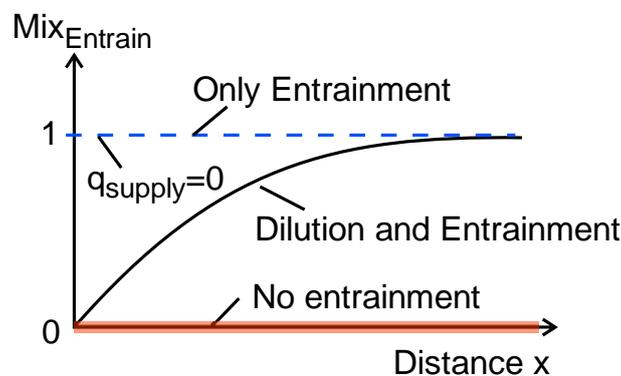
Figure 2. The mixing factor due to entrainment as a function of distance from the supply
