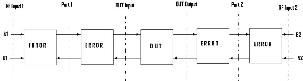
Figure 14 : Error model for calibration.
