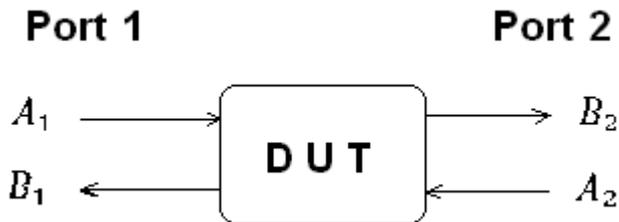
Figure 1 : Waves at Port 1 and Port 2 of a DUT (Device under Test).
