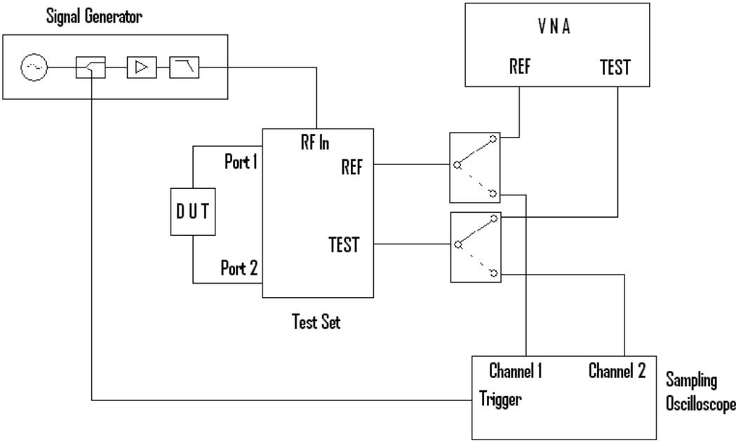
Figure 7 : Measurement system using sampling oscilloscope and a VNA.
