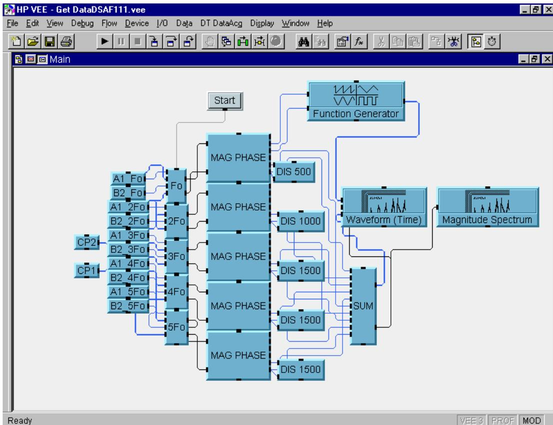
Figure 27 : Programming module for final computation of time domain waveform
