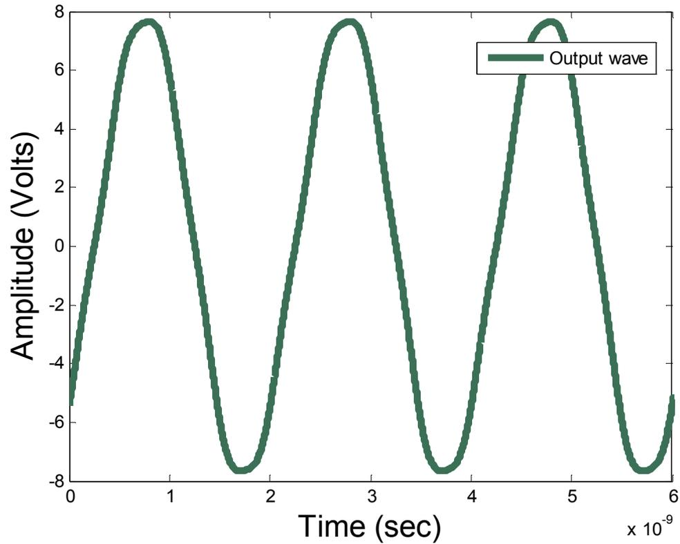
Figure 22 : Measured output wave for 3dBm input by internal source to ZHL-2-8 (DUT 2)
