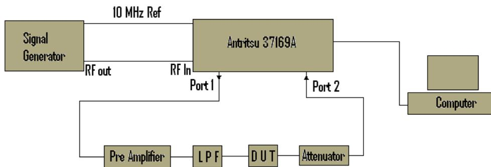
Figure 18 : Architecture of designed measurement system.
