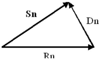
Figure 11 : Vector diagram for measured signal by VNA.
