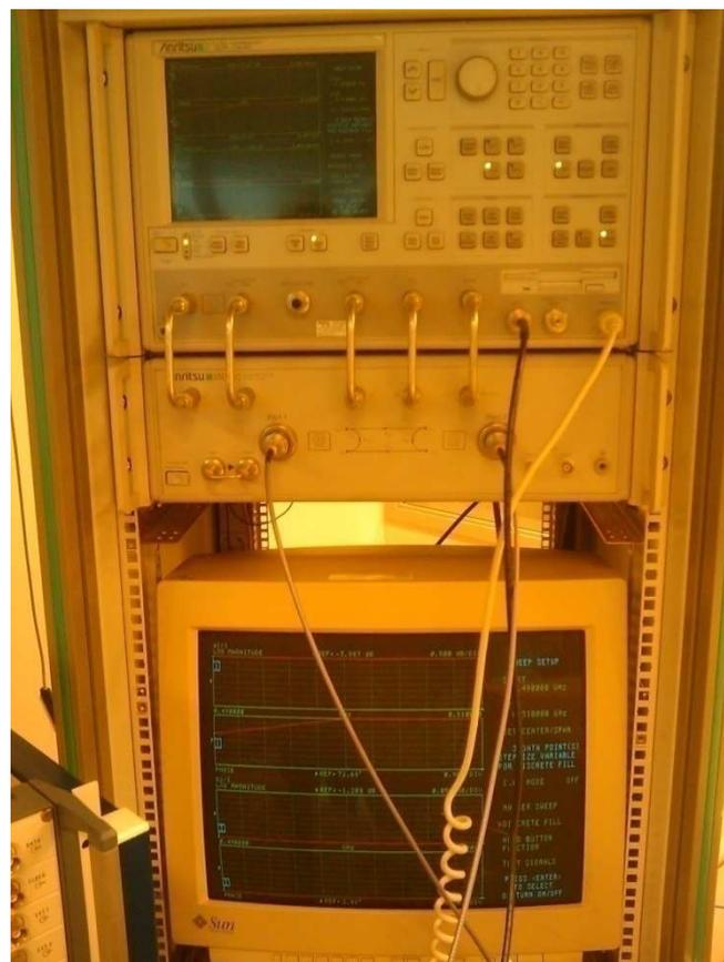
Figure 19 : Anritsu 37169A that was used as a tuned receiver
