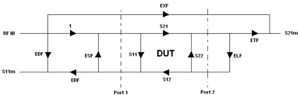
Figure 4 : 6 -Term Error Model (One path Two Port Calibration).
