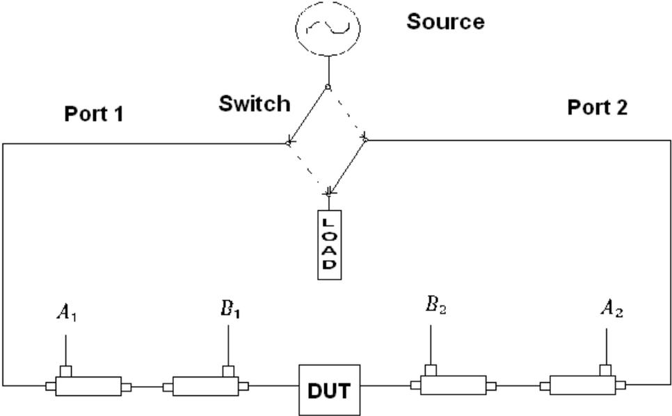
Figure 8 : Source and Signal separation unit in a typical VNA.
