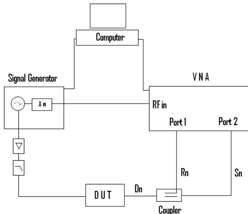
Figure 10 : Measurement System a VNA.
