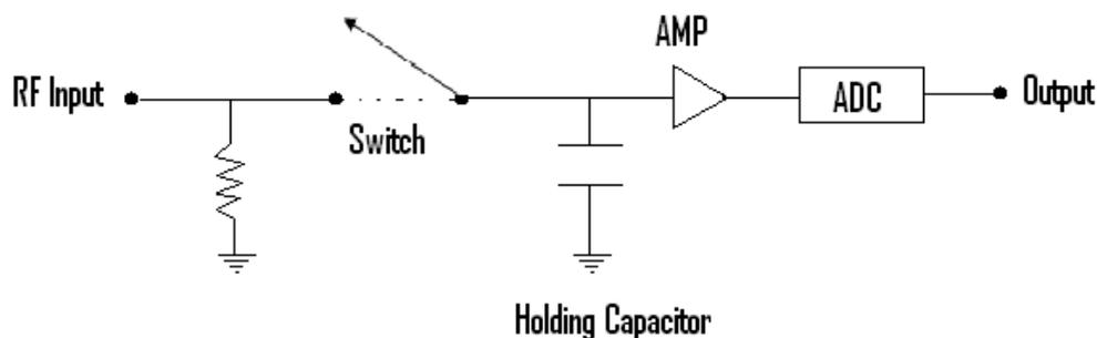
Figure 5 : Sampler Circuitry for sampling oscilloscope.
