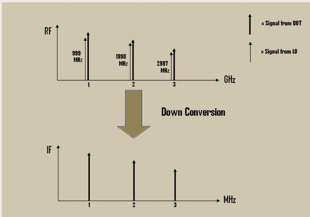
Figure 17 : Harmonic mixing of LO with input Spectrum.
