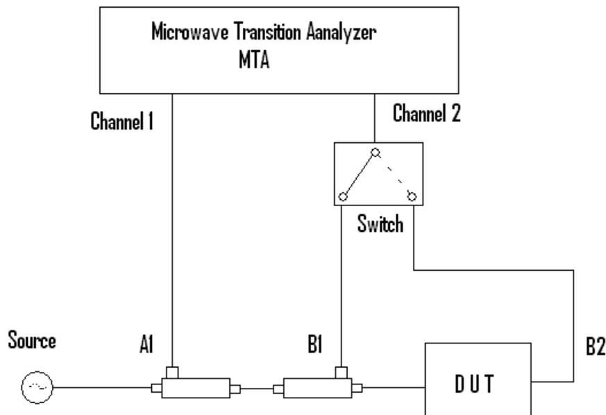
Figure 15 : Measurement system using MTA.
