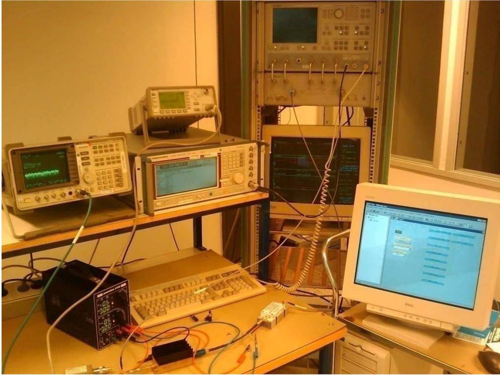
**Figure 20 : Implemented Large Signal RF Measurement System using a tuned receiver**
