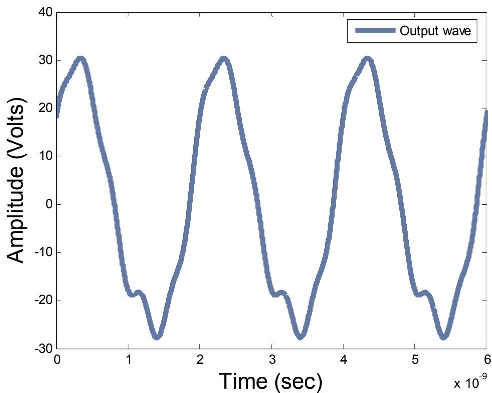
Figure 21 : Measured output wave for 3dBm input by internal source to ZHL-42 (DUT 1)
