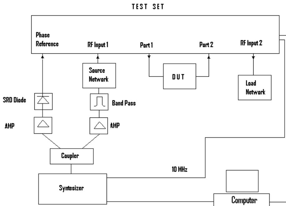
Figure 12 : Block Diagram of measurement system using VNA in receiver mode.
