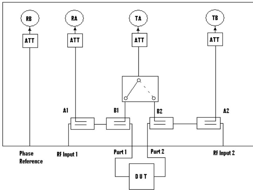
**Figure 13 : Modified test set configuration.**
