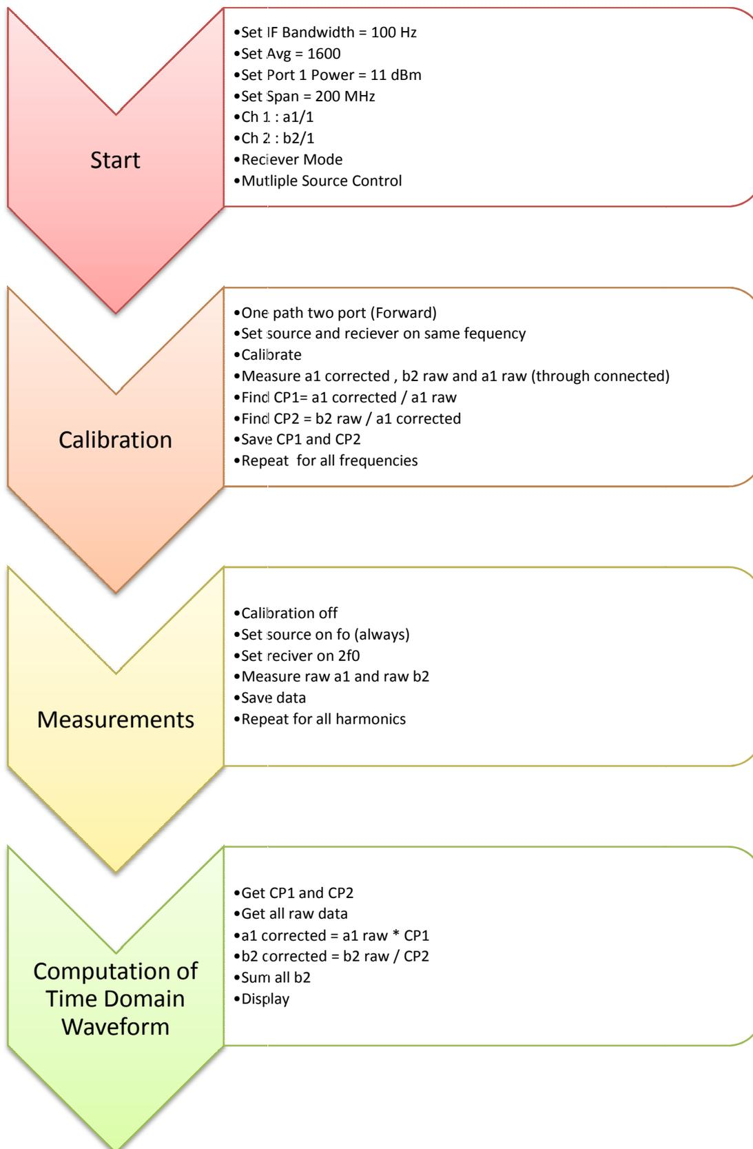
Figure 25 : Flow diagram for measurement system using a tuned receiver
