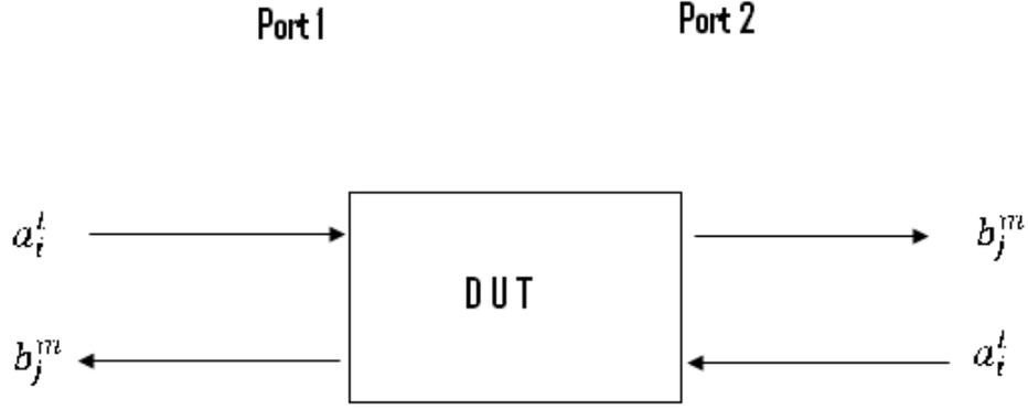
Figure 3 : Two port nonlinear network.
