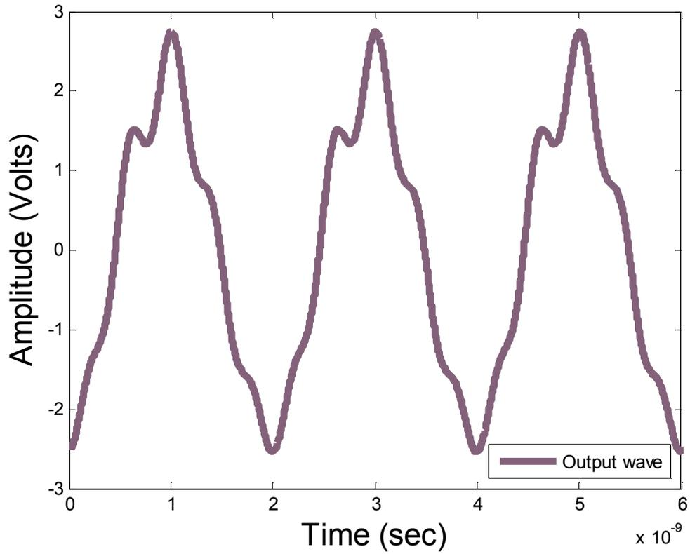
Figure 23 : Measured time domain waveform of 3dBm signal by internal source
