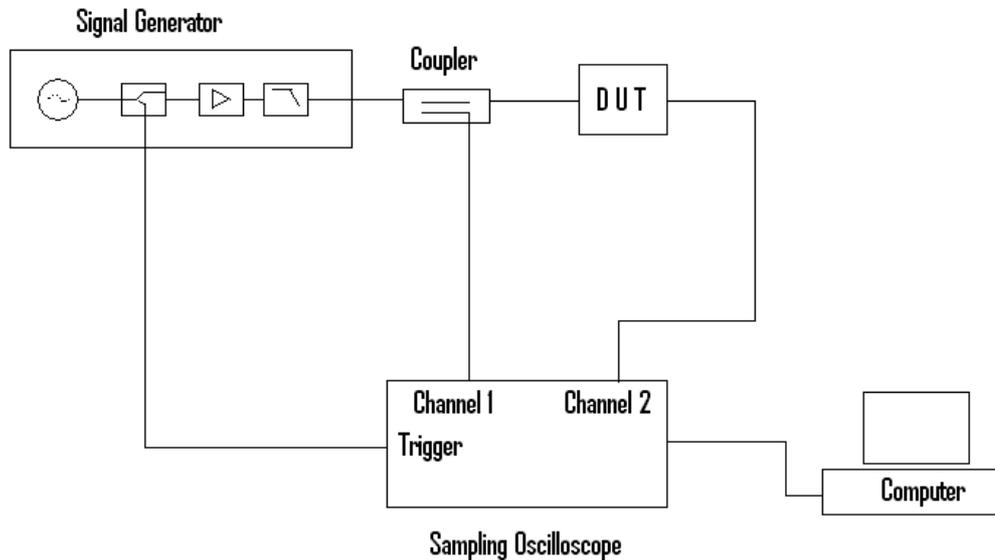
Figure 6 : Measurement system using sampling oscilloscope.
