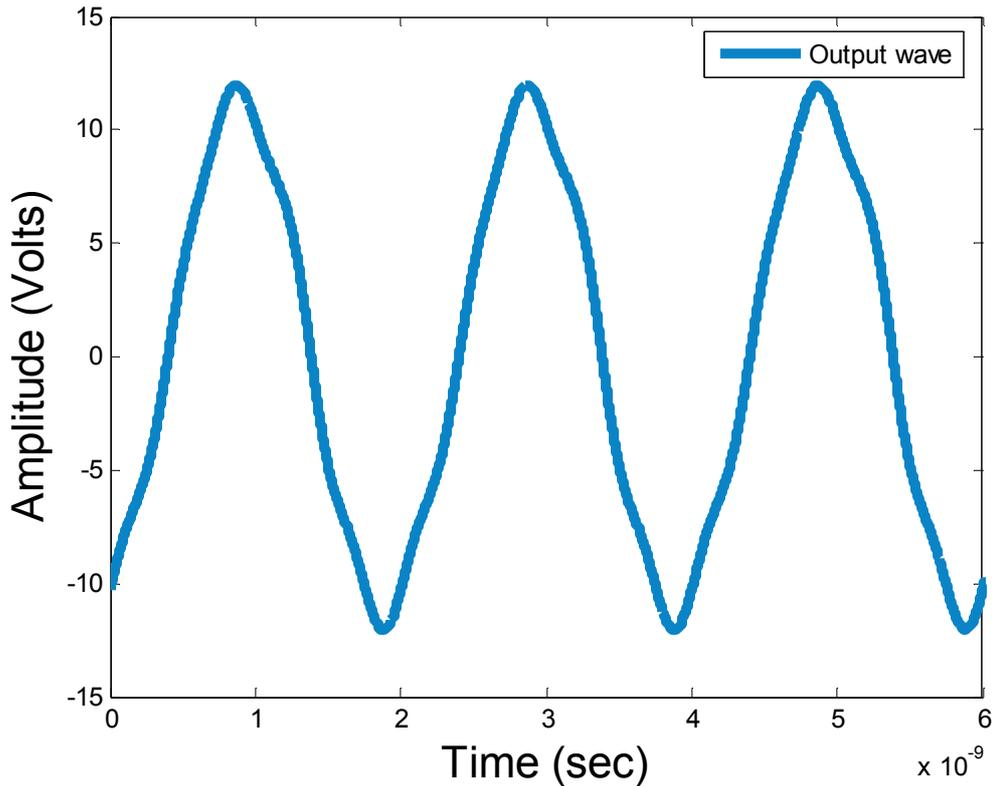
Figure 24 : Measured output wave for 3dBm input by external source to ZHL-2-8 (DUT 2)
