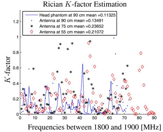
**Figure 4.**  $K$ -factor of a reverberation chamber with no stirrers where  $S_{21d}$  equals mean of the  $S_{21i}$  samples, horizontal receiving dipole.
