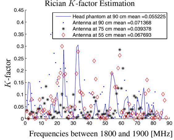
**Figure 3.**  $K$ -factor of a reverberation chamber with no stirrers where  $S_{21d}$  equals mean of the  $S_{21i}$  samples, vertical receiving dipole.
