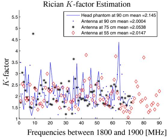
**Figure 5.**  $K$ -factor of a reverberation chamber with no stirrers where  $|S_{21d}|$  equals mean of the magnitudes of the  $S_{21i}$  samples.
