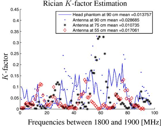
**Figure 1.**  $K$ -factor of a stirred reverberation chamber where  $S_{21d}$  equals mean of the  $S_{21i}$  samples, vertical receiving dipole.
