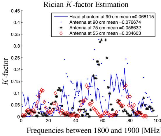
**Figure 2.**  $K$ -factor of a stirred reverberation chamber where  $S_{21d}$  equals mean of the  $S_{21i}$  samples, horizontal receiving dipole.
