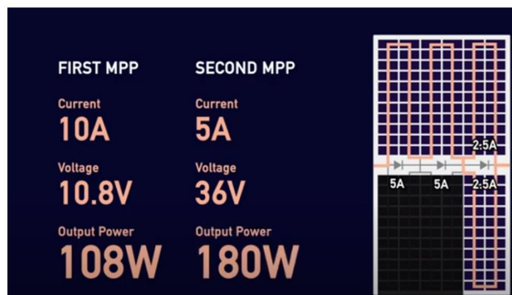
FIGURE 9 MULTIPLE MPPS EFFECT ON POWER OUTPUT (GSES, 2021)
