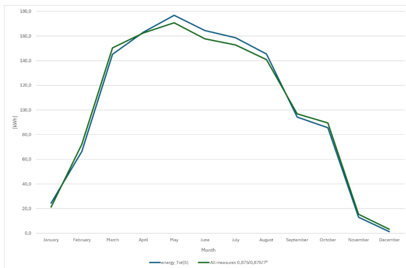
FIGURE 15: WINSUN PV RESULTS COMPARED TO MEASUREMENTS 2 (HERNANDO URIARTE, 2024)
