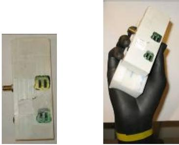
Fig. 2 PIFA prototype in freespace and in hand
