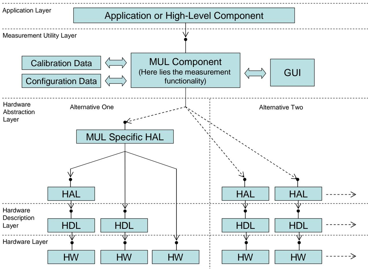
Fig. 2. The proposed SW structure of the VI measurement system. High-level programs, such as test programs, HPVVEE, Labview, etc., resides in the Application Layer. The measurement functionality resides in the MUL. The HAL makes the MUL and Application Layer HW agnostic, while the HDL contains HW communication.
