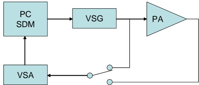
Fig. 8. The HW set-up of the implemented VI measurement system.
