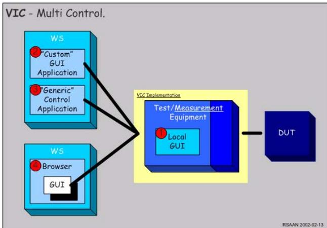
Fig. 6. The concept of multi control. The VIC supports the simultaneous access from several different applications.
