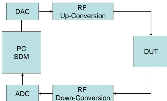
Fig. 7. Principle for the general HW set-up for RF measurements.
