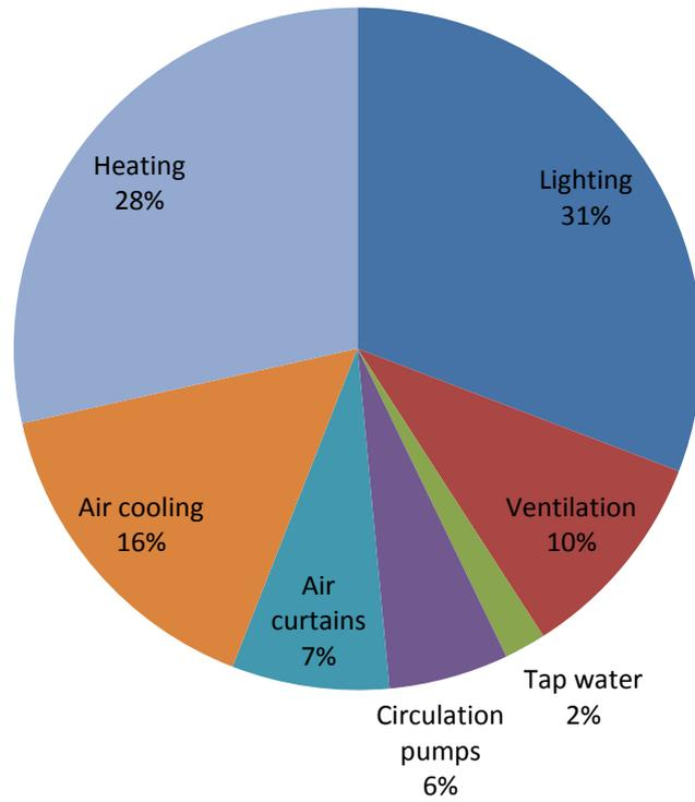
Figure 11. Electricity consumption in support processes
