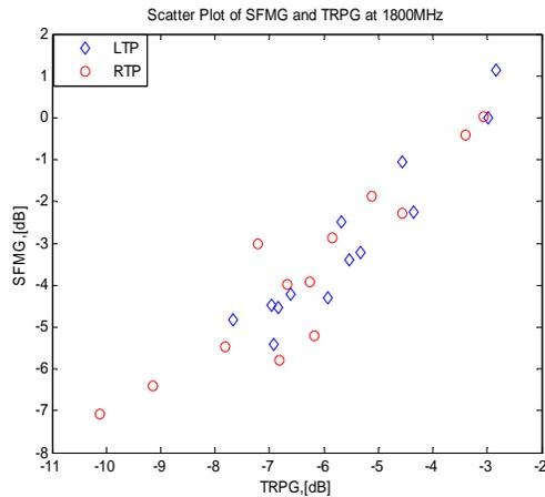
**Figure 9 - TRPG vs.SFMG at 1800 MHz for 13 measured phones**
