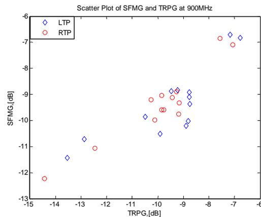
Figure 8 - TRPG vs. SFMG at 900 MHz for 13 mobile terminals
