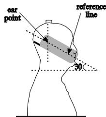
Figure 3 - Phantom with Handset in talk position
