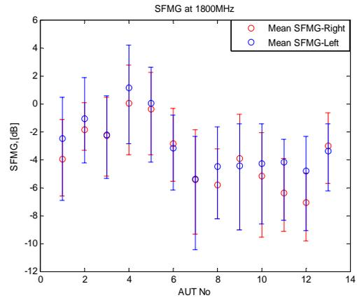
Figure 7 - SFMG at 1800 MHz vs. AUT No.
