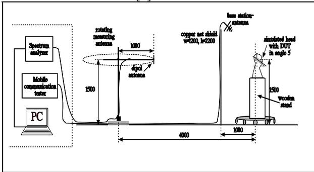
**Figure 1 - Arrangement of test equipment. Note: Handset speaker centered at ear and above centre of turntable**
