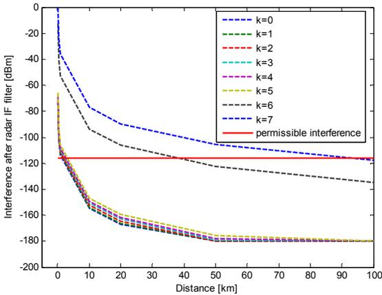
Figure 4b: Interference at the victim L band radar receiver injected by an adjacent channel apart by  $\pm k$  channels from the radar operating channel.
