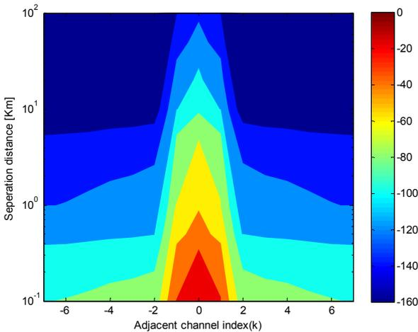
Figure 5a. Interference at the victim S band radar receiver as a function of spatial and frequency separation of k channels from the radar system.
