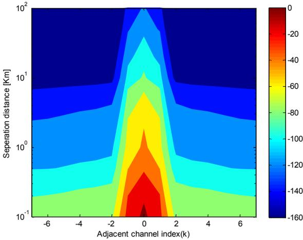
Figure 4a: Interference at the victim L band radar receiver as a function of spatial and frequency separation of k channels from the radar system.
