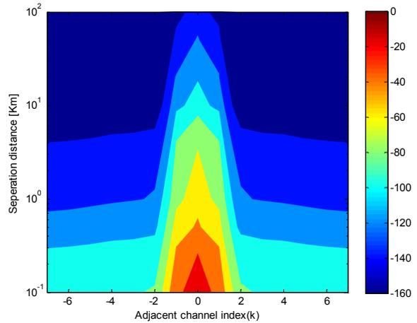
Figure 6a. Interference at the victim C band radar receiver as a function of spatial and frequency separation of k channels from the radar system.
