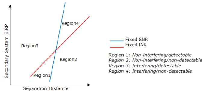
Figure 2. Regions of detect-ability and interfere-ability as functions of SS EIRP and separation distance
