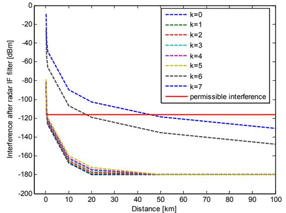
Figure 6b. Interference at the victim C band radar receiver injected by an adjacent channel apart by  $\pm k$  channels from the radar operating channel.
