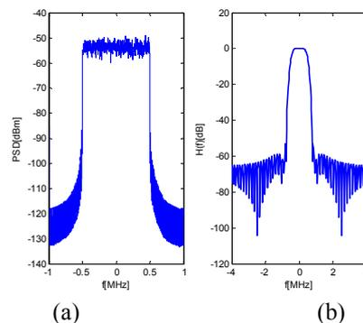
Figure 3. (a) Normalized SS OFDM baseband spectra and (b) The radar magnitude filter response.
