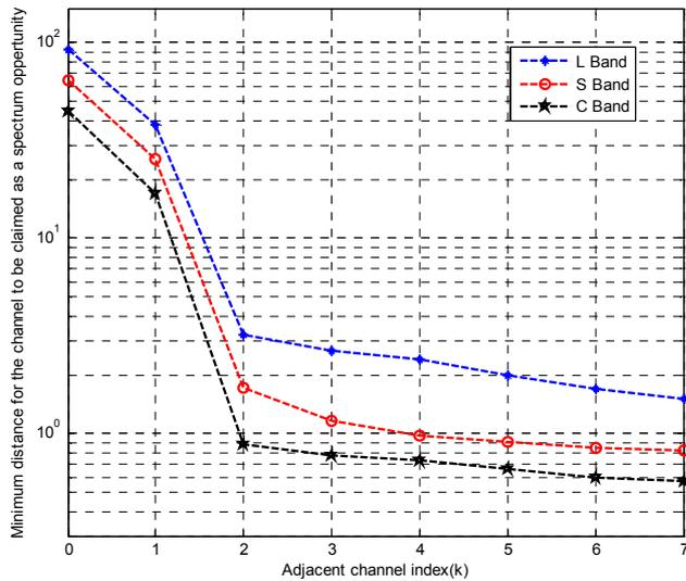
Figure 7. Minimum distances from the radar receiver to the SS to occupy a channel apart by  $\pm k$  from the radar channel
