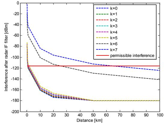
Figure 5b. Interference at the victim S band radar receiver injected by an adjacent channel apart by  $\pm k$  channels from the radar operating channel.
