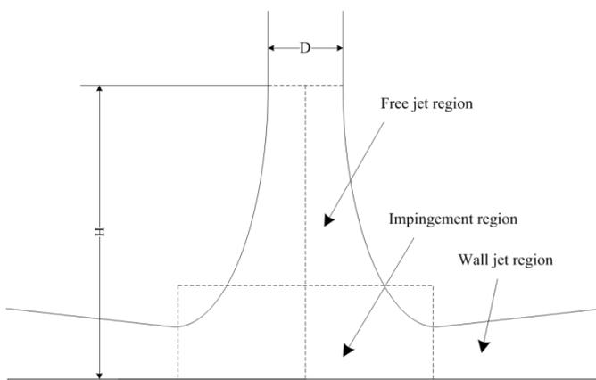
Figure 1. Flow regions of an impinging jet
