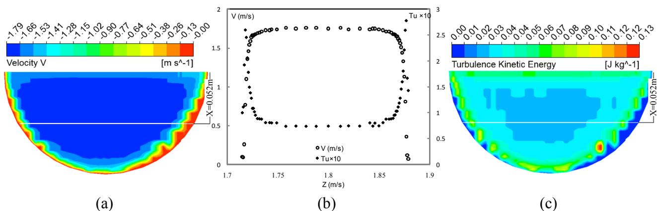
Figure 5. Boundary conditions for the velocity profile,  $V$ , (a) and the turbulence kinetic energy profile (c) used for the numerical simulation based on the measured values at 4 mm beneath the supply exit section of the impinging jet. (b): the represented measured velocity  $V$  and turbulence intensity  $T_u$  profiles at a distance of  $0.052$  m from the bottom of the pipe.
