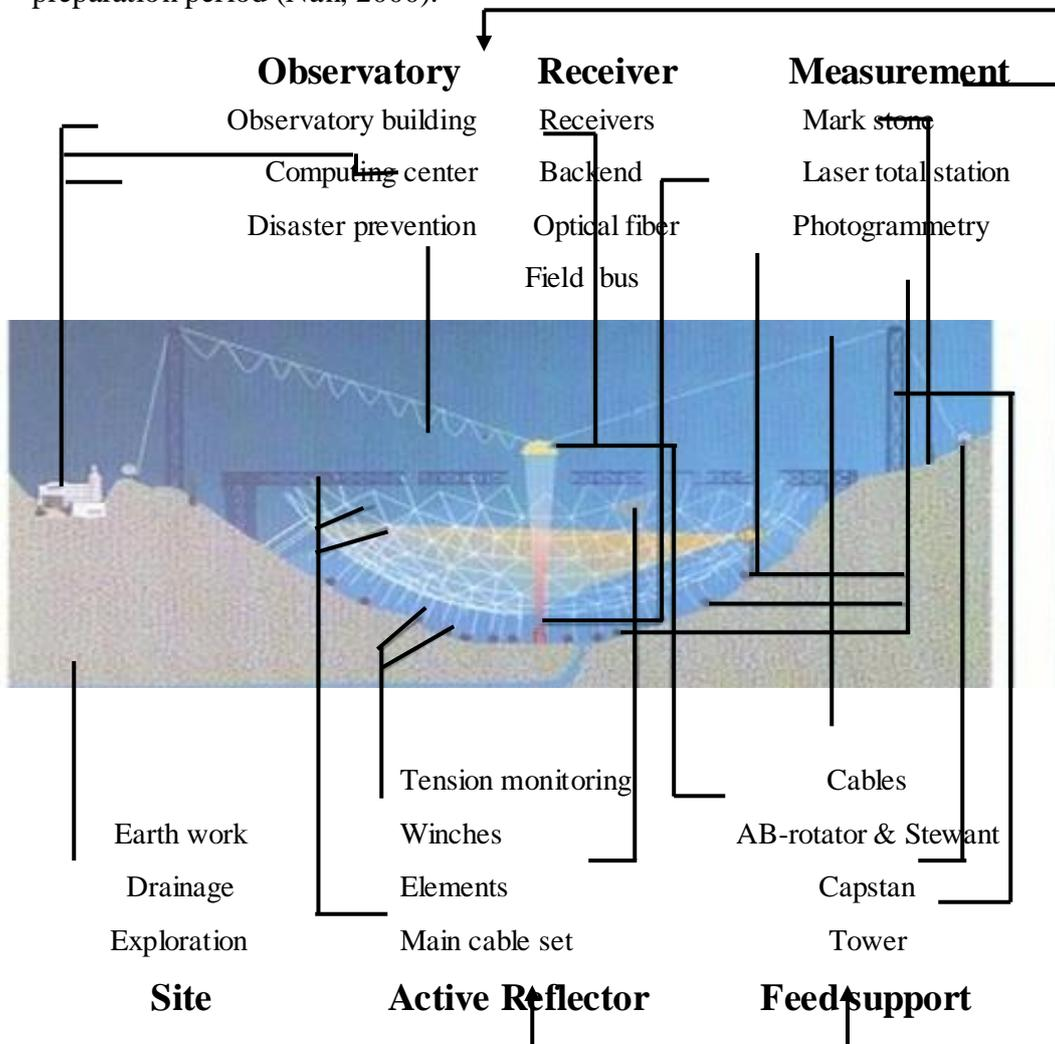
Figure 12: The sub-system of FAST
