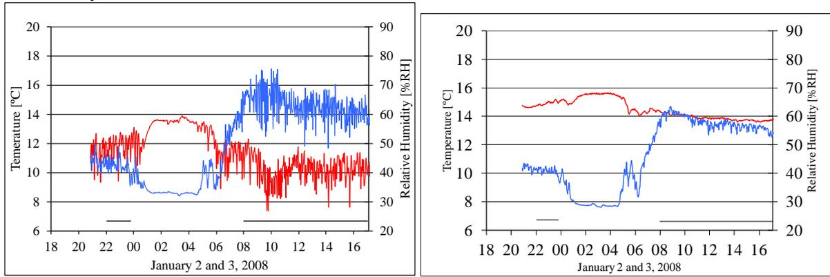
Figure 2. Temperature (red) and relative humidity (blue) in ticket hall X (left) and ticket hall Y (right). Measuring periods are marked.
