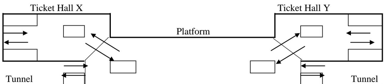
Figure 1. Schematic design of the underground station. The ticket halls are in direct contact with the outside air. On either side of ticket halls, the tunnels are in contact with the outside air via ventilation shafts. Therefore the platform may receive fresh air either via the ticket halls or the tunnels.
