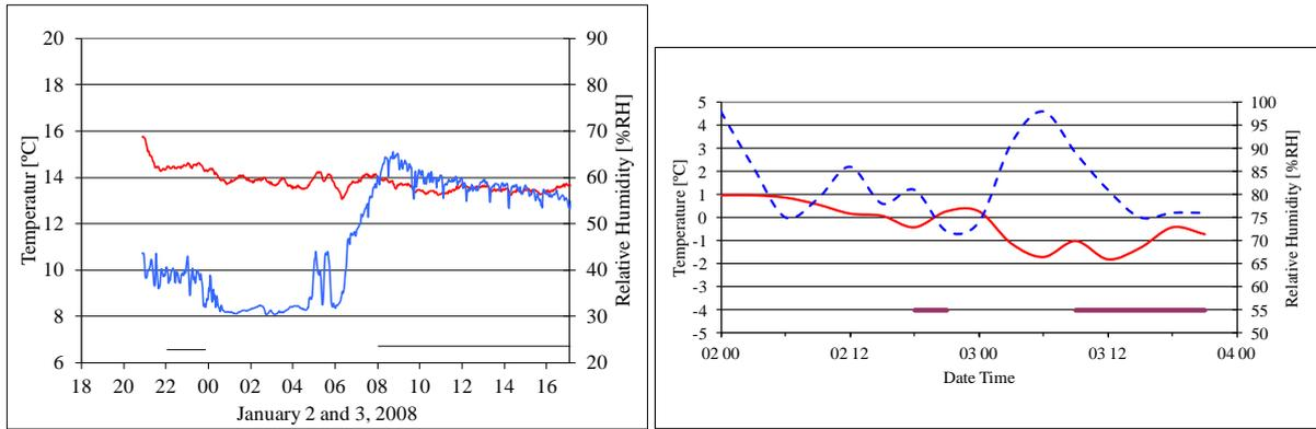
Figure 3. Temperature (red) and relative humidity (blue) in the middle of the platform (left) and outdoors (right). The measuring periods are marked.
