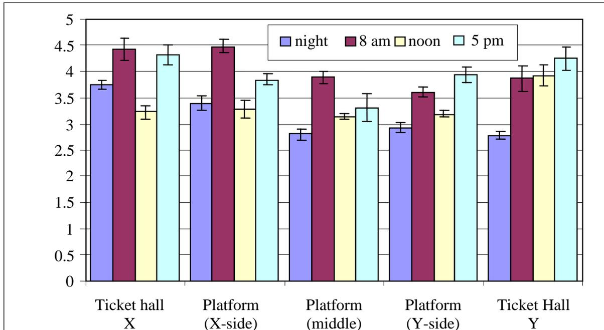
Figure 5. The local air change rate, ACH ( $\text{h}^{-1}$ ) measured at selected points for all the measuring periods (see legend). The error bars are also given.
