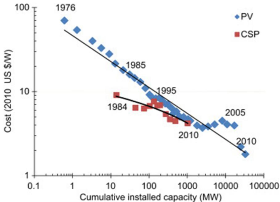
**Figure 8.** PV modules between 1976 and 2010, CSP systems between 1984 and 2010 [14]
