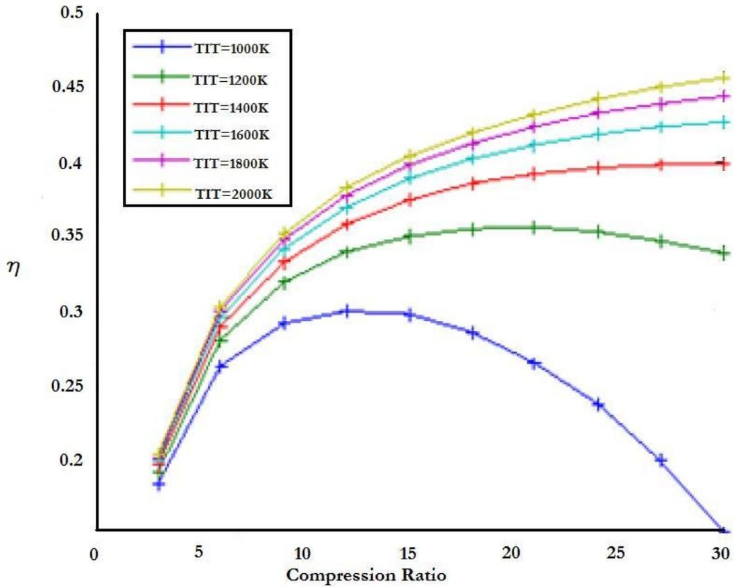
Figure 8: Variation of compression ratio and turbine inlet temperature on thermal efficiency (Rahman, et al., 2011)
