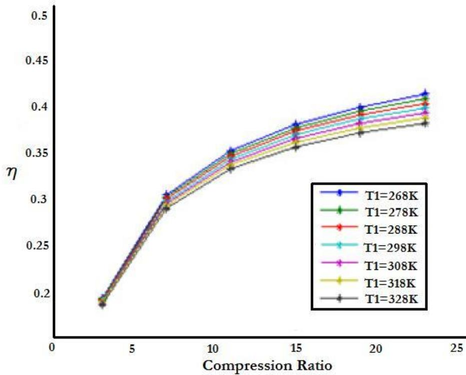
Figure 9: Variation of compression ratio and ambient temperature on thermal efficiency (Rahman, et al., 2011)
