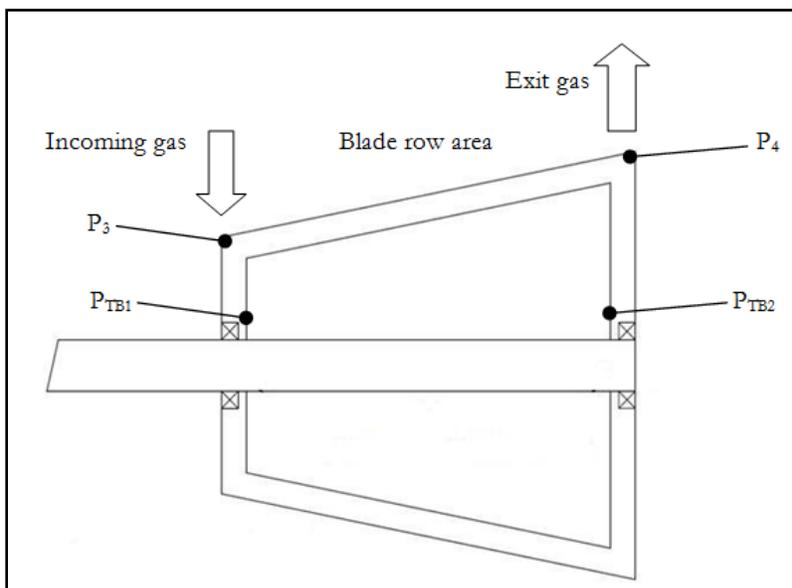
**Figure 30:** The pressure values in the turbine
