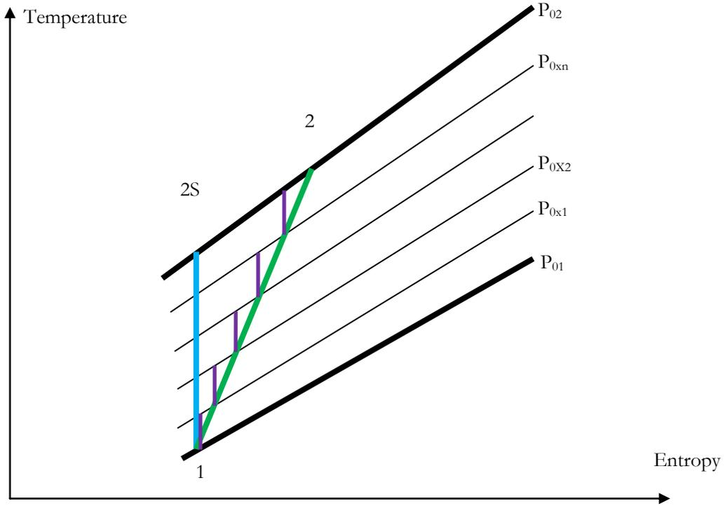
Figure 14: T-S diagram for compression process
