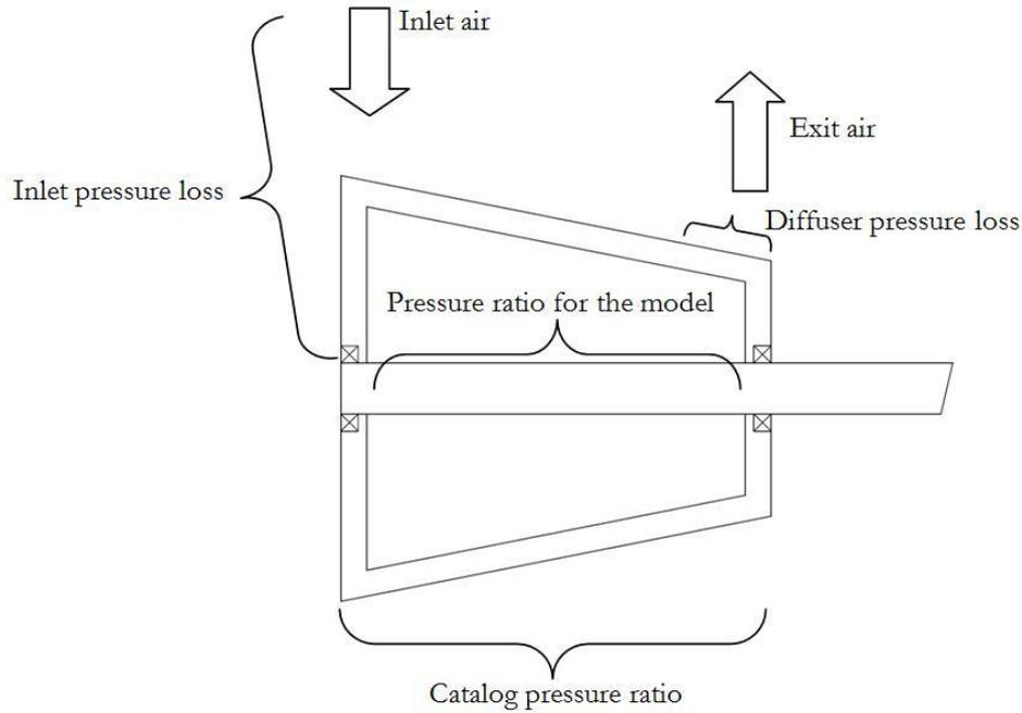
Figure 15: Pressure losses and pressure ratios in the compressor
