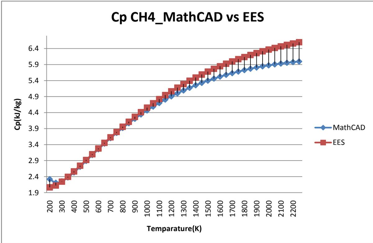
Figure 20: Difference between the Cp (Mathcad) and Cp(EES) for Methane (200K-2250K)
