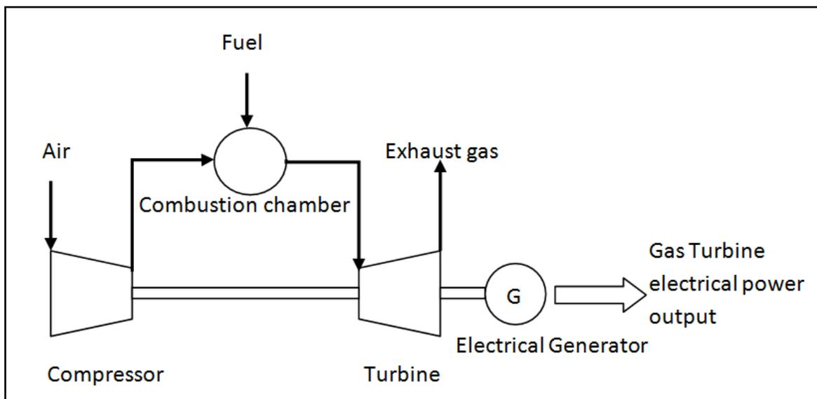
*Figure 23: Typical open gas turbine*
