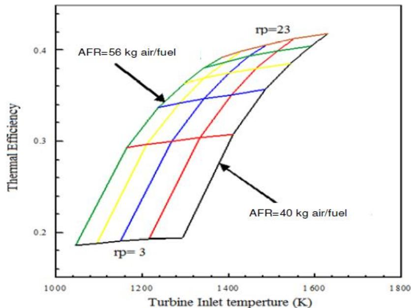
Figure 10: Variation of turbine inlet temperatures with thermal efficiency for several compression ratio and air to fuel ratio (Rahman, et al., 2011)
