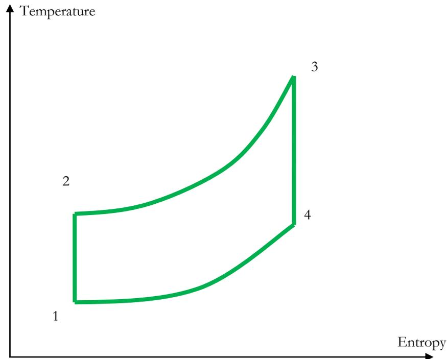
Figure 2: T-S diagram for closed gas turbine cycle
