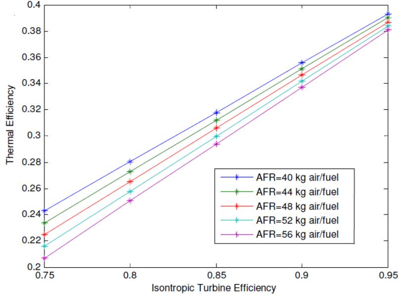
Figure 12: Effect of isentropic turbine efficiency air to fuel ratio on thermal efficiency. (Rahman, et al., 2011)
