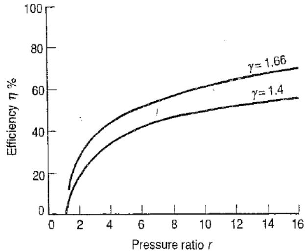
Figure 7: Relation between pressure ratio and efficiency. (Cohen, et al., 1996)
