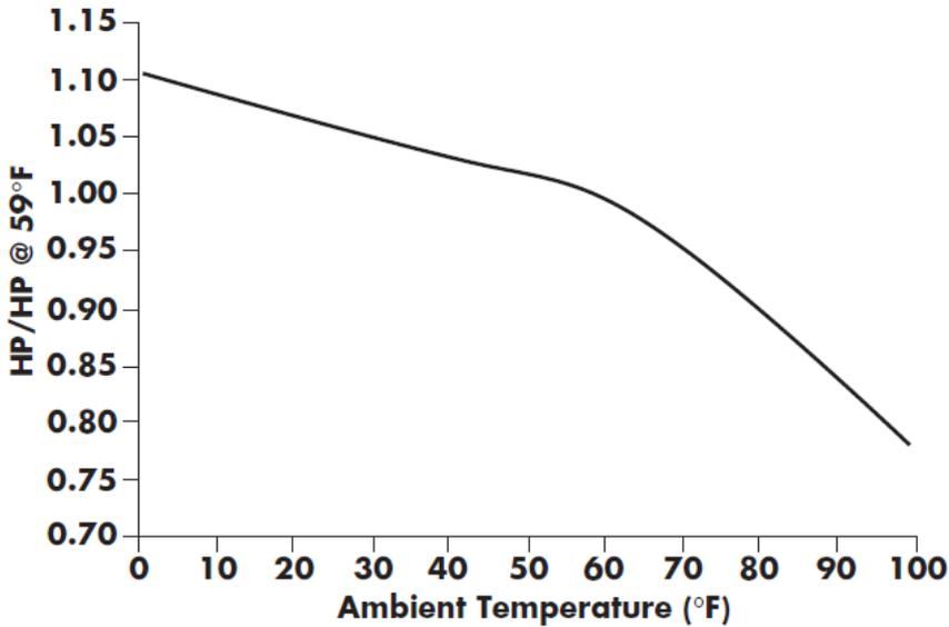
Figure 3: Ambient Temperature Power Correction Factor Curve (Petchers, 2002)
