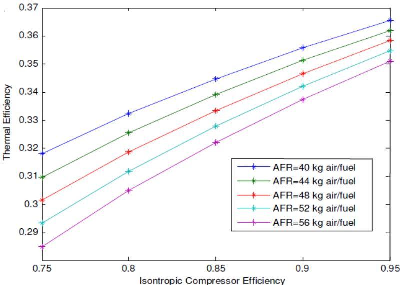
Figure 11: Effect of isentropic compressor efficiency air to fuel ratio on thermal efficiency. (Rahman, et al., 2011)
