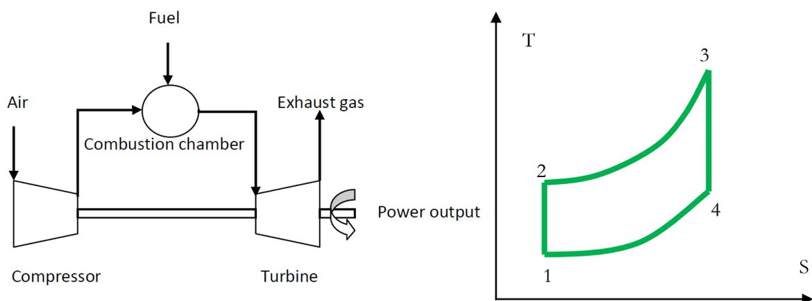
Figure 6: Open gas turbine and T-S diagram
