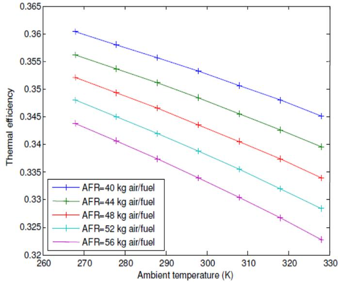
Figure 4: Effect of ambient temperature and air to fuel ratio on thermal efficiency (Rahman, et al., 2011)
