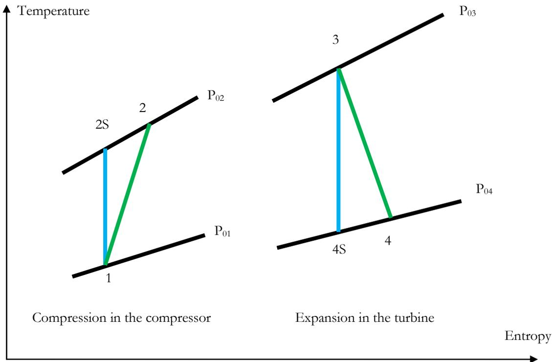
Figure 13: T-S diagram for compression and expansion
