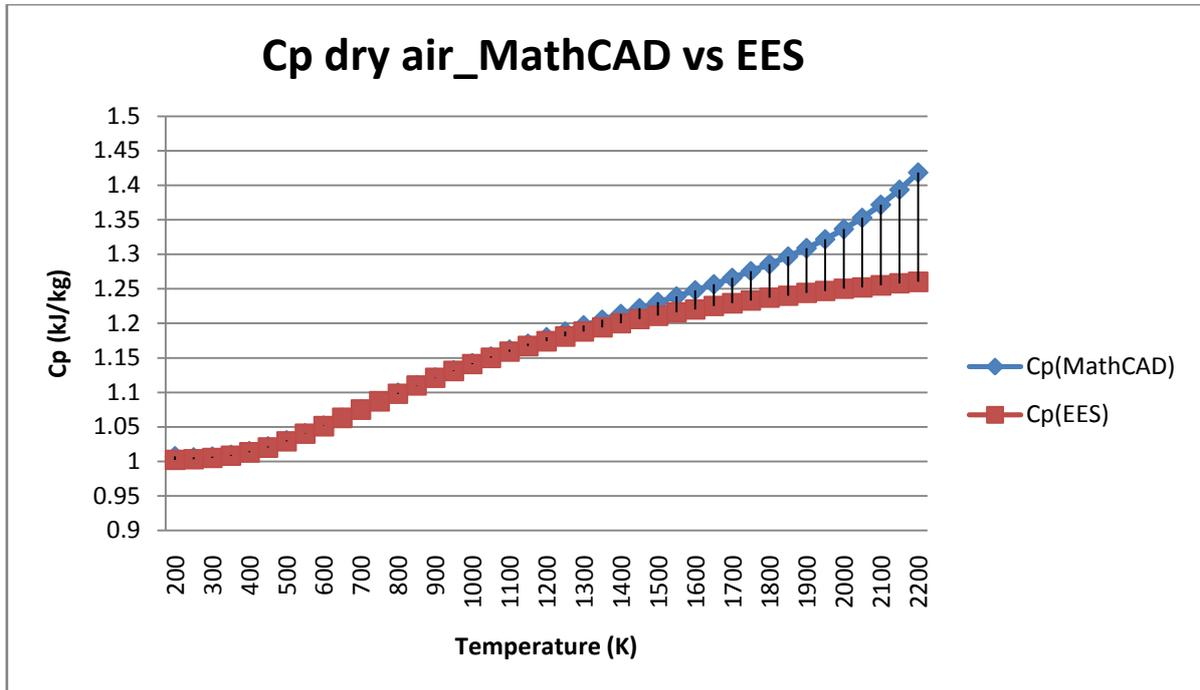
Figure 19: Difference between the Cp (Mathcad) and Cp(EES) for dry air (200K-2150K)
