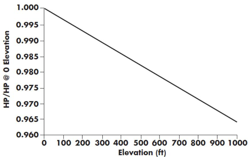
Figure 5: Representative Altitude Power Correction Factor Curve
