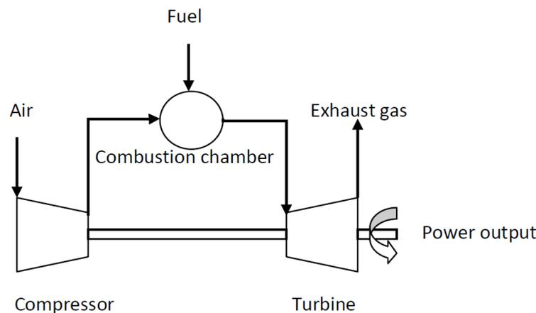
Figure 1: Typical open gas turbine
