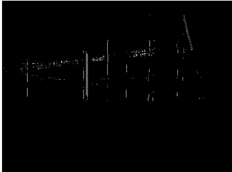
*Figure 9 Vertical line extraction with Hough*
