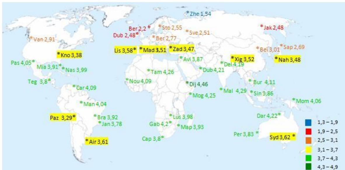
**Fig. 6: Ratio Flat plate 50°C to PV 14.6% polycrystalline**
