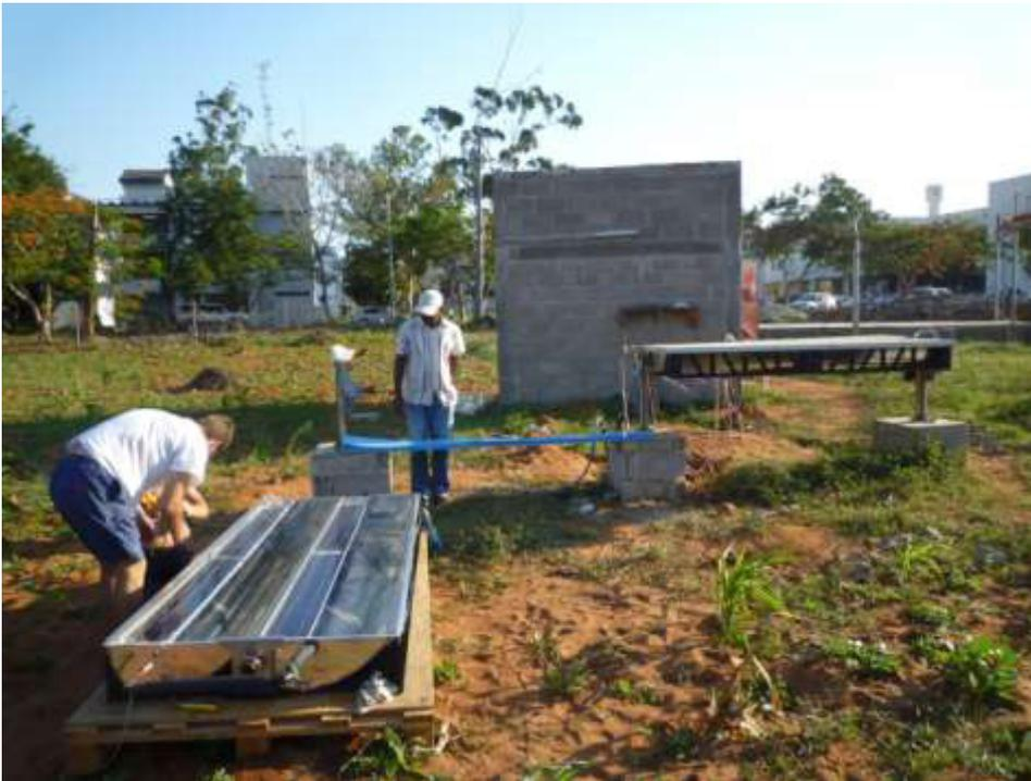
Fig. 2. Testing of a photovoltaic / thermal hybrid collector in front of the solar laboratory. The laboratory is located at the Universidade Eduardo Mondlane in Maputo, Mozambique.
