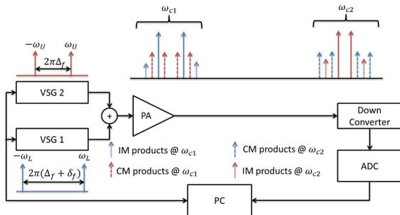
Fig. 1. Measurement setup for the characterization of concurrent dual-band power amplifier [2].
