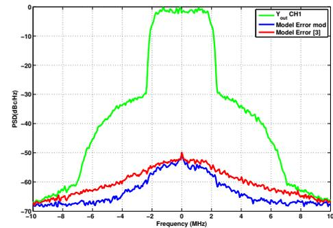
Fig. 3. Signal spectrum (green) and error spectra for the original model (red) and the model modified based on the result from the dual two-tone test [2].
