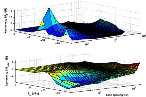
Fig. 2. Asymmetric energy surface between lower-upper IM products (top). Asymmetric energy surface between lower-upper CM products (Bottom) [2].
