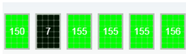
Figure 10. Power in Wp from each panel of system 2, in the case where two cells shaded. Each square represents the PV panel and the number inside is its power output in W.
