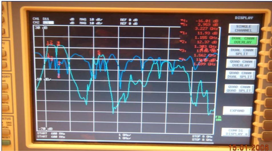
**Figure-6.10 The Gain and input return loss response of implemented RF front end**
