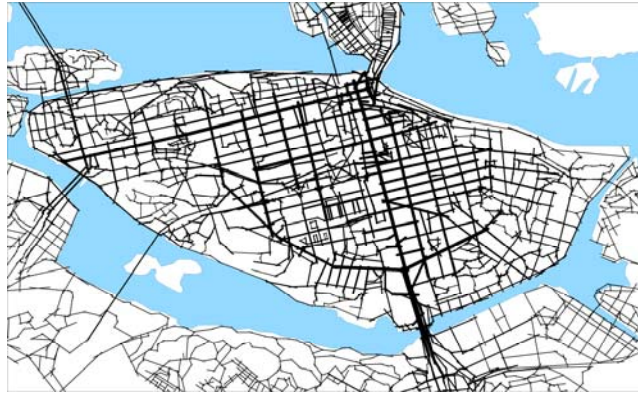
Fig. 3. The distribution of spatial integration, correlating in this case with observed pedestrian movement by 70% (R 2 =0.70)
