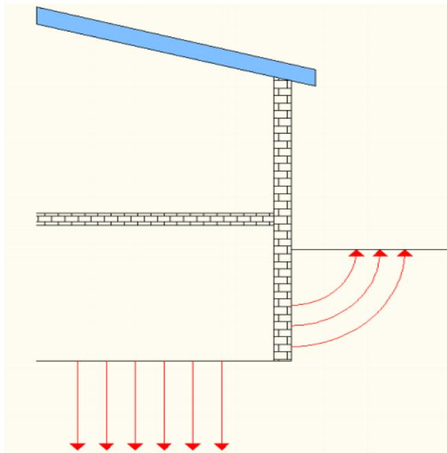
*Figure 2.5 Different way of transmission through floor and wall[11]*
