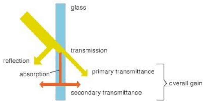
Figure 2.8 Solar radiation through the window[21]
