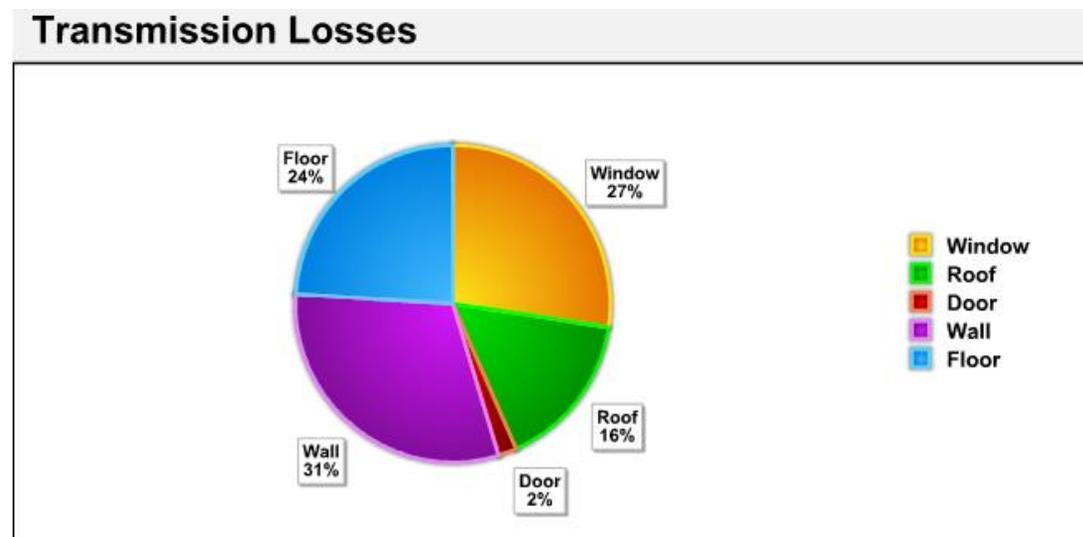
*Figure 4.3 Transmission losses*
