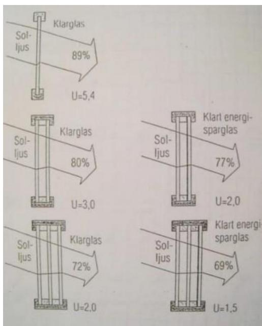
Figure 2.10 The U-value and factor of different windows[7]
