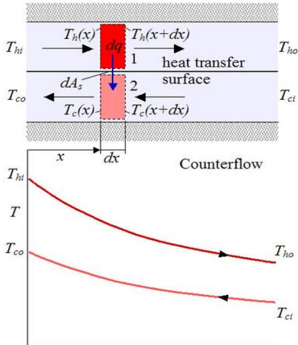
Figure 2.4. A schema of a counter flow exchanger[23]
