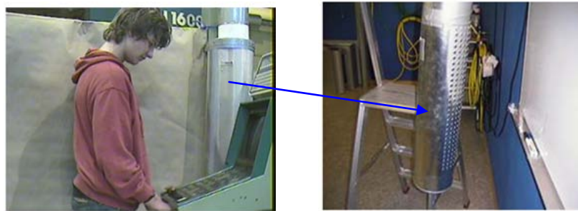
Figure 1. Confluent jets supply device blowing towards worker with expanded metal.
